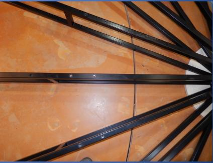
The longest distance from the bolt hole to the end should be towards the centre.
